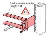
2 Slide the TPG 262 into the rack chassis adapter ...
