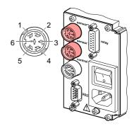
Pin assignment of the two female 6-pole Amphenol C91B appliance connectors:
